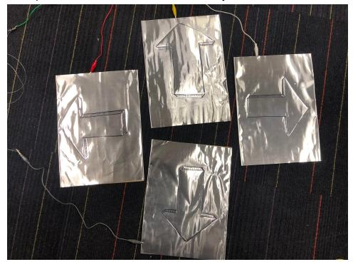
• Makey-Makey. Each footpad is connected to the corresponding key on the Makey-Makey. The ground is connected to the handle.
